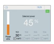
Temperature Mode keeps the PCBA at a selected temperature, using the regulation or protection TC.
