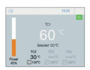
Profile Mode allows control of the heating rate of the PCBA by the use of a control and a protection thermocouple.
