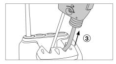
Place the cartridge in the quick tip changer extractor and pull the tool to remove the cartridge (3).
