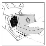
Remove the wiper by pulling it out.
