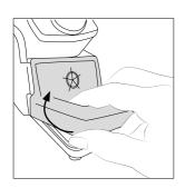
Lift the wiper at its front edge.
