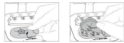
Replace the wool for a new one and reassemble the wiper. Make sure that the wiper is correctly inserted all around
