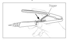
Lower the trigger until it gets locked into one of the grooves of the plunger.
