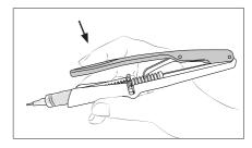
Press the lever until solder paste comes out.
