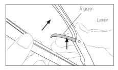
Open DPM by lifting the lever and the trigger.
