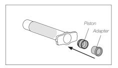
Take the barrel filled with solder paste and place the piston into the barrel.
