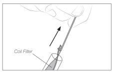
Remove the coil filter, check the filter and replace it if it is dirty or damaged.
