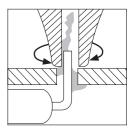
Press the vacuum pump button long enough to remove the solder.
