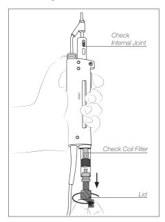
The lid must be unscrewed with the DR560 in a vertical position.
