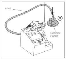
Connect the hose of the fume aspiration duct to the collector flange FAE030 or FAE040 (3). The flanges must be connected to the fume extractor.
