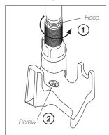
First remove the hose by twisting it (1). Shake the hose to get rid of the dirt inside.
