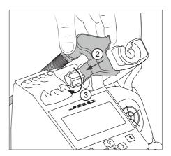
Insert the fume aspiration duct between the knob and the tool holder (2).
