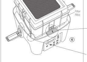
**Note:** The main filter has a given position. Make sure the filter ribs mate with the corresponding slots.
