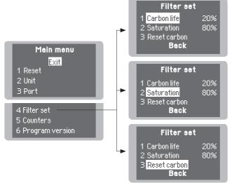
Shows % of remaining life of the carbon filter contained inside the FAE1-100 filter. It is also displayed on the main screen.
