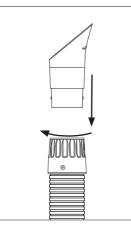
To install a new nozzle, turn the nozzle bayonet clockwise to lock it in place.
