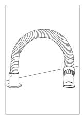
The arm can be used by placing the nozzle over the solder joint or resting it on the work surface.
