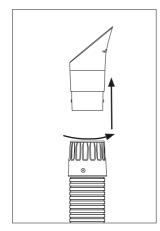
The bayonet system makes it easy to change the nozzle. To do this, hold the tube with one hand and with the other turn the nozzle counter-clockwise and pull it out to remove the nozzle.
