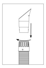
The bayonet system makes it easy to change the nozzle. To do this, hold the tube with one hand and with the other turn the nozzle counterclockwise and pull it out to remove the nozzle. To install a new nozzle, turn the nozzle bayonet clockwise to lock it in place.
