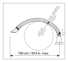
To avoid breaking the arm, do not extend the arm more than 100 cm / 39.4 inches from the center of its base and do not go below the minimum bend radius of 20 cm / 7.87 inches.
