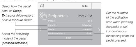
\*NB: The same can be applied reversely by continuously pressing the pedal and releasing to activate.
