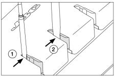
C210 cartridges are held between the internal clamps (1) and C245 cartridges between the external clamps (2).
