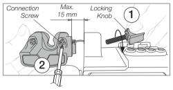
Using a flat-blade screwdriver, guide the cable connector outward to completely detach the support from the station.  $\triangle$  Any force exerted for extraction must be applied on the connector, never on the cable.
